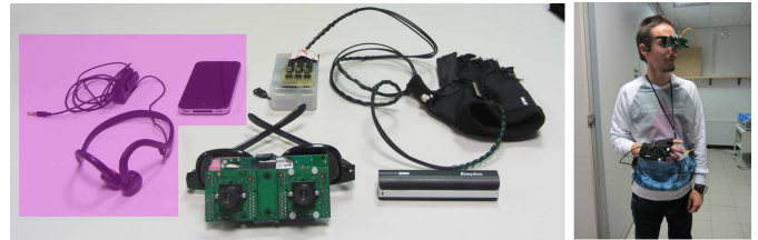
Fig. 2. On the left, hardware components of the proposed mobility aid: custom RGBD camera ( \approx 90 g with lenses and holders), embedded computing platform ( \approx 50 g), glove with micro-motors for tactile feedback (few grams), the pocket battery ( \approx 70 g), bone-conductive headset ( \approx 45 g) and smartphone. In purple, the optional components. On the right, the overall system worn by a user.
