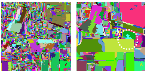
Figure 1. Tsukuba (portion of the reference image R): superpixels obtained by means of (Left) over-segmentation and (Right) relaxing over-segmentation. The circle highlights a superpixel overlapping a depth discontinuity (table/background).
