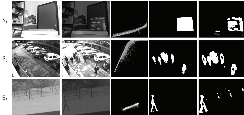
Fig. 2. Qualitative results yielded by the proposed algorithm on the 3 test sequences. For each sequence, from left to right: the inferred background, one sample frame, the joint intensity histogram, the ground truth mask and the binary change mask.
