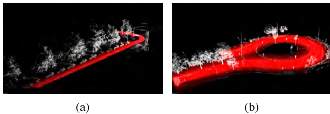
Fig. 3: Road pavement detection and removal (red points). The point clouds come from the Oakland 3-D Point Cloud Dataset (left) and our urban dataset (right); for details see Sec. III.
